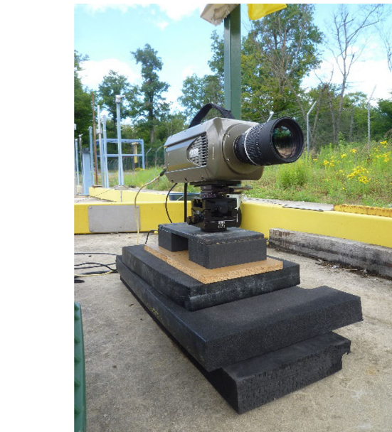
Fig. 7 High-speed camera used during ISL tests (V310 Phantom camera)
