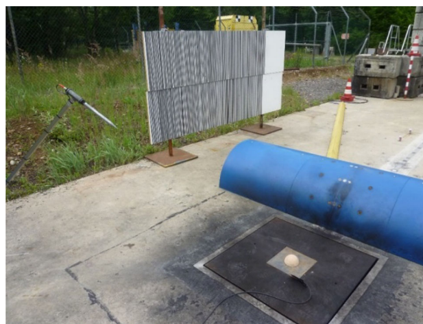
Fig. 5 ISL experimental setup with a 333-g Hexomax® charge—53 cm between the charge and hemicylinder
