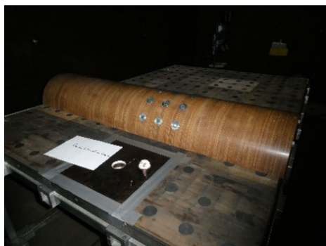
Fig. 3 IRSN experimental setup with a 41.5-g Hexomax® charge—27 cm between the charge and hemicylinder
