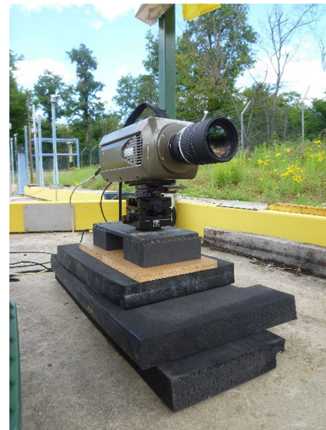
Fig. 7 High-speed camera used during ISL tests (V310 Phantom camera)
