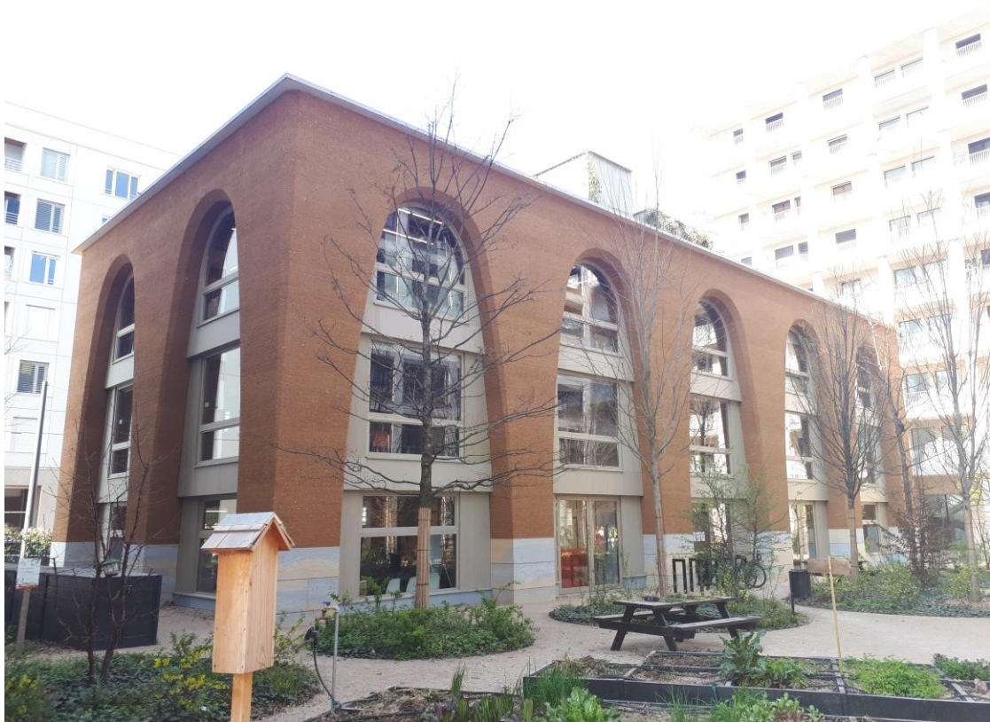
Figure 1: L'Orangerie, building in Lyon, dated 2019 made of pre-fabricated rammed earth.
