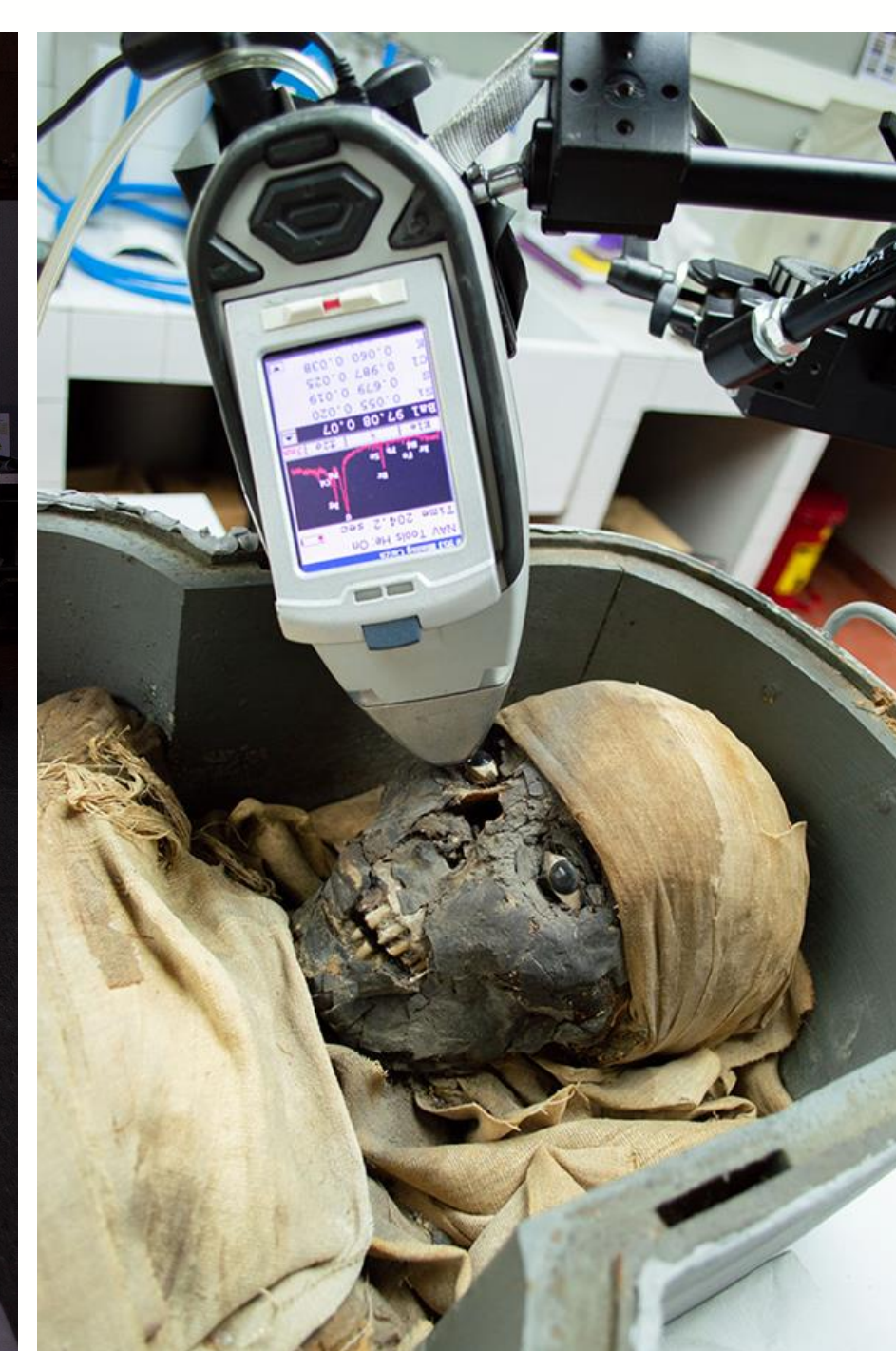
XRF analysis on the artificial eyes of Setjaimengaou © C2RMF/V. Fournier
