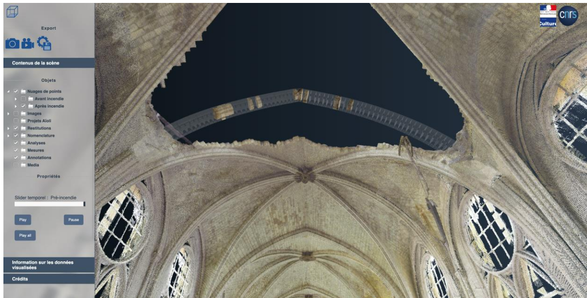
Fig. 6. Virtual anastylosis of the voussoirs of the collapsed arch in the nave of the cathedral, displayed in the NDP 3D Viewer.
