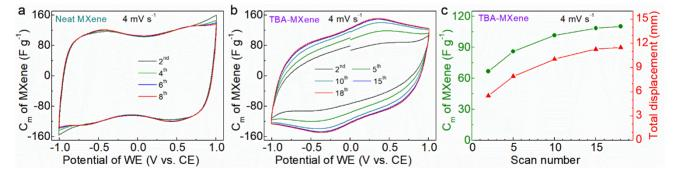
**Figure S6**. Supplemental data of the ECAs working in a 5.6 M LiBr solution electrolyte (as shown in Figure S3). (a,b) CV curves at 4 mV  $\rm s^{-1}$  of (a) neat MXene and (b) TBA-MXene based ECAs. (c) Evolution of the specific capacitance and total displacement of TBA-based ECA during the CV measurement at 4 mV  $\rm s^{-1}$ .
