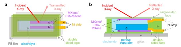
**Figure S10**. Illustration of in-situ XRD tests of neat MXene and TBA-MXene films in two-electrode cells. (a) The transmission mode for the (110) peak. A Nickel plate (thickness:  $\sim 0.1$  mm) was covered on the counter electrode (the lower one) to block its (110) signal. (b) The reflection mode for the (002) peak. The porous poly(vinylidene difluoride) separator (pore size: 0.22 mm; thickness:  $\sim 0.1$  mm) was confirmed effective for blocking the (002) signal of the bottom electrode.
