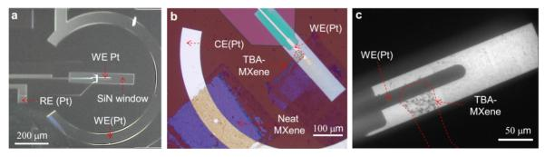
**Figure S13**. Set-up for in situ electrochemical liquid cell TEM experiments. (a, b) Optical images of the electrochemical chip (a) before and (b) after sample transfer (red dotted rectangle). (c) Low-magnification TEM image of the transferred sample (red dotted line).
