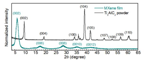
Figure S1. XRD pattern of the neat MXene film and the Ti<sub>3</sub>AlC<sub>2</sub> powder.
