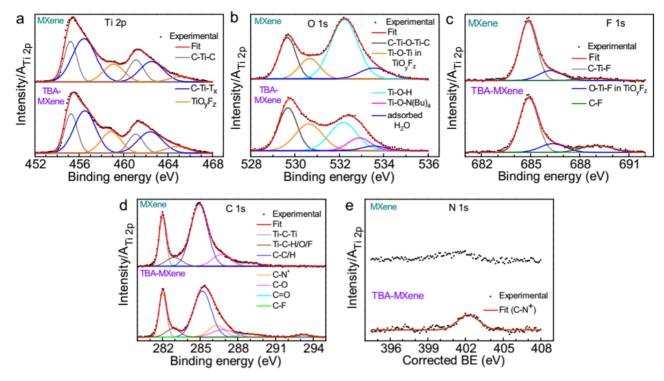
**Figure S5**. Deconvoluted (a) Ti 2p (T denotes terminal groups such as –O, -OH, -OLi, -O-TBA, -F and -Cl), (b) O 1s, (c) F 1s, (d) C 1s, and (e) N 1s XPS spectra of the neat MXene and TBA-MXene films. The intensity of all spectra is normalized to the area of the Ti<sub>2p</sub> peak.
