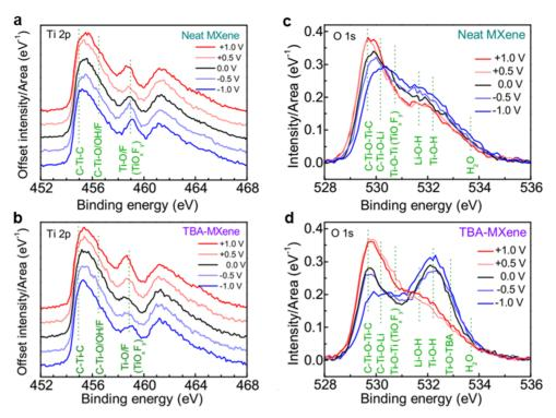
**Figure S12.** Ex-situ XPS spectra of the working electrode (WE) films after charging to different potentials vs. the counter electrode (CE): (a, b) Normalized Ti 2p survey; (c, d) Normalized O 1s survey.
