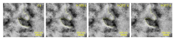
**Figure S14**. Sequential TEM images of TBA-MXene sheets in the liquid cell before applying a potential. The yellow dotted line indicates the position of the profile at t s. The sheets are stable under irradiation for more than 5 min.
