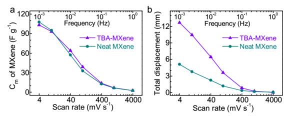
**Figure S16**. Comparison of the specific capacitance and total displacement of IECAs based on neat MXene and TBA-MXene under different scan rates. The free length was 17 mm.
