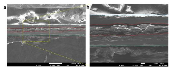
**Figure S15**. SEM images of the cross-section of a TBA-MXene based IECA before infiltration of the liquid electrolyte. Red dotted lines mark the interface between the TBA-MXene film and the TPU/CMF paper.
