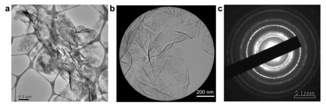
Figure S2. (a, b) TEM images and (c) corresponding selected area electron diffraction pattern of aggregated TBA-MXene sheets in (b).
