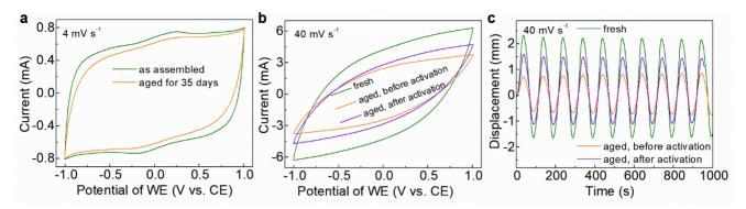
**Figure S18**. Effect of aging in ambient condition (21 °C, 65% relative humidity) on the performance of TBA-MXene based ECA: (a) CV curves at 4 mV s<sup>-1</sup> before and after 35-day aging; (b) CV curves at 40 mV s<sup>-1</sup> before and after 35-day aging. The activation was done by running a CV at 4 mV s<sup>-1</sup> for 10 cycles; (c) Actuation displacement of fresh and aged device at 40 mV s<sup>-1</sup> under a triangle wave of  $\pm$  1V and 0.01 Hz.
