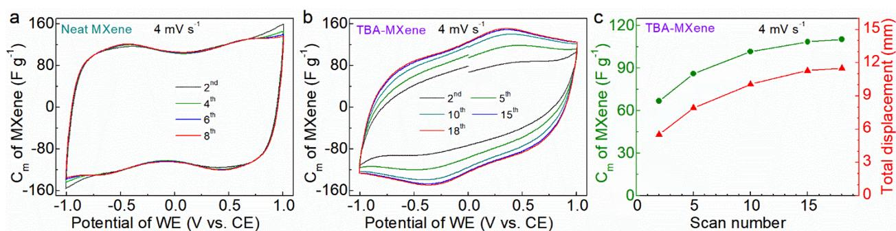
**Figure S6.** Supplemental data of the ECAs working in a 5.6 M LiBr solution electrolyte (as shown in Figure S3). (a,b) CV curves at  $4 \text{ mV s}^{-1}$  of (a) neat MXene and (b) TBA-MXene based ECAs. (c) Evolution of the specific capacitance and total displacement of TBA-based ECA during the CV measurement at  $4 \text{ mV s}^{-1}$ .
