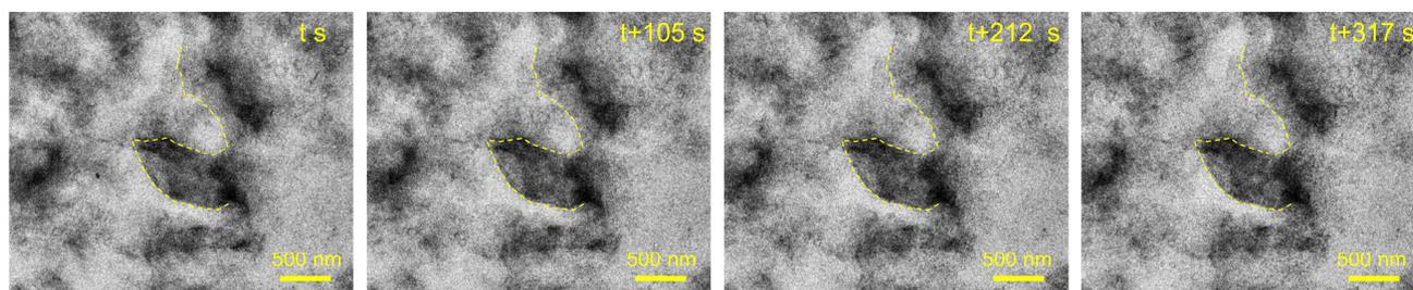
**Figure S14.** Sequential TEM images of TBA-MXene sheets in the liquid cell before applying a potential. The yellow dotted line indicates the position of the profile at  $t$  s. The sheets are stable under irradiation for more than 5 min.
