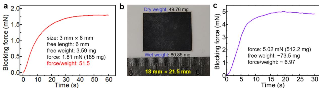
**Figure S17.** Performance of short and wide IECAs: (a) Blocking force of a short IECA (free length = 6 mm) under DC 1 V for 30 s. (b, c) Photo and blocking force of a wide IECA under DC 1 V for 30 s.
