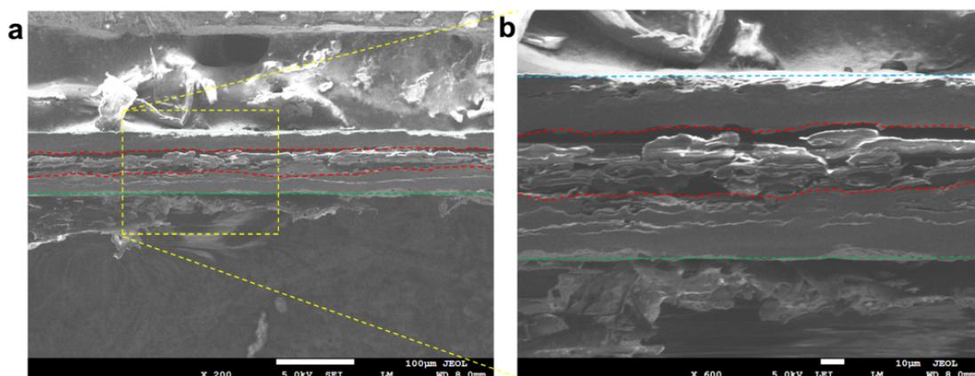
**Figure S15.** SEM images of the cross-section of a TBA-MXene based IECA before infiltration of the liquid electrolyte. Red dotted lines mark the interface between the TBA-MXene film and the TPU/CMF paper.
