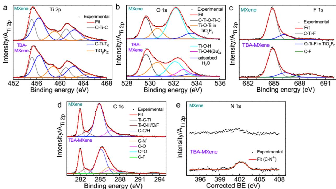
**Figure S5.** Deconvoluted (a) Ti 2p (T denotes terminal groups such as  $-O$ ,  $-OH$ ,  $-OLi$ ,  $-O-TBA$ ,  $-F$  and  $-Cl$ ), (b) O 1s, (c) F 1s, (d) C 1s, and (e) N 1s XPS spectra of the neat MXene and TBA-MXene films. The intensity of all spectra is normalized to the area of the  $Ti_{2p}$  peak.
