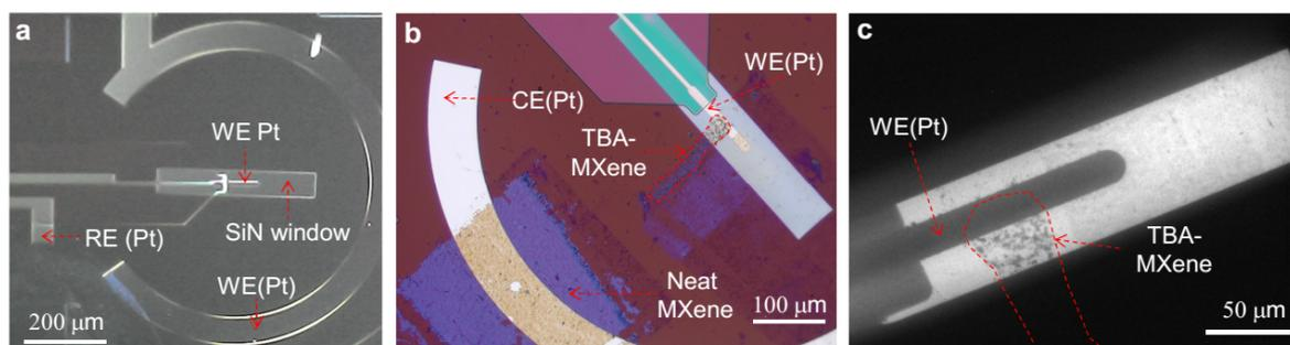
**Figure S13.** Set-up for in situ electrochemical liquid cell TEM experiments. (a, b) Optical images of the electrochemical chip (a) before and (b) after sample transfer (red dotted rectangle). (c) Low-magnification TEM image of the transferred sample (red dotted line).
