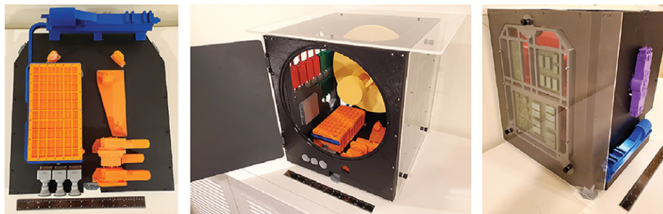
Fig. 3. A half-scale printed model of the TOMCAT payload demonstrates fit and assembly of the SmallSat ESPA Grande package. (left) The laser (orange) is attached to the bottom panel of the instrument. (center) The telescope (yellow) and detectors (red and green) are shown in the fully assembled instrument, while (right) the electronics cards are shown on the side panel. The panels are clear in this 3D printed model, but the actual panels are made of M55J composite over an aluminum core.
