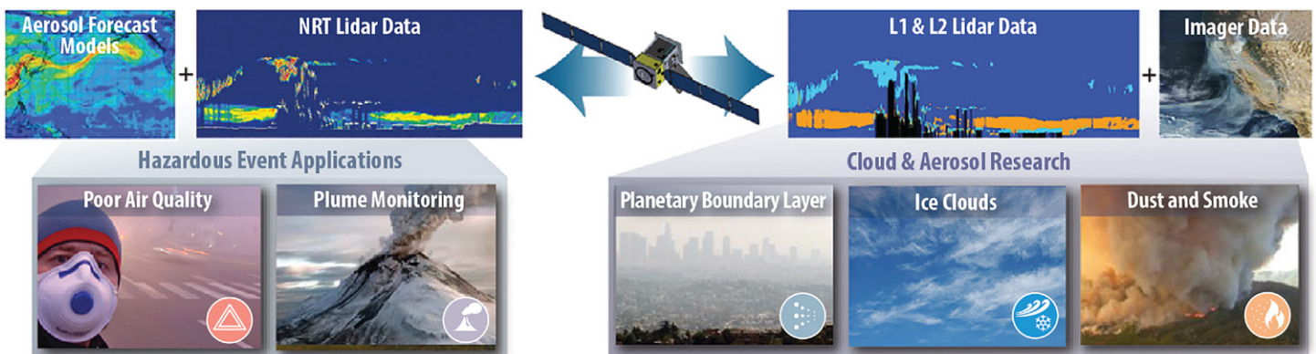
Fig. 1. Near-real-time lidar data products from TOMCAT, combined with aerosol forecast models, enable air quality forecasting and hazardous plume monitoring applications. The TOMCAT lidar and multiangle imager provide the data products necessary to achieve science objectives that advances our understanding of the diurnal and seasonal variability of aerosols, clouds, and PBL vertical structure. Icons (bottom-right corners in each panel of the second row) are used throughout the paper to highlight the mission’s five themes/objectives.
