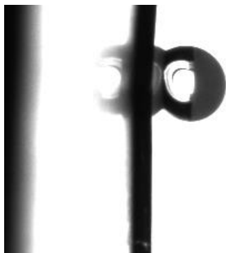
Figure 7. Example of water droplet on our surfaces with an inclination angle of 90°.
