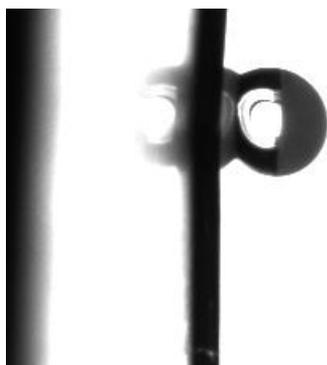
**Figure 7.** Example of water droplet on our surfaces with an inclination angle of  $90^\circ$ .
