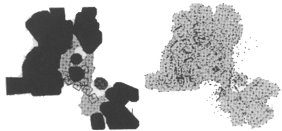
Fig. 11. The model of Fig. 10 after obstacle growing (left) and the nodes defined by the region segmentation (right).
