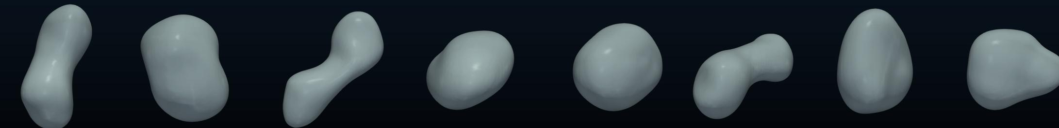
Droplet breakup under turbulent conditions is not such a straight-forward process. A series of droplets initialized on a spherical state surrounded by a turbulent flow were realized and left to evolve until breakup was reached.
