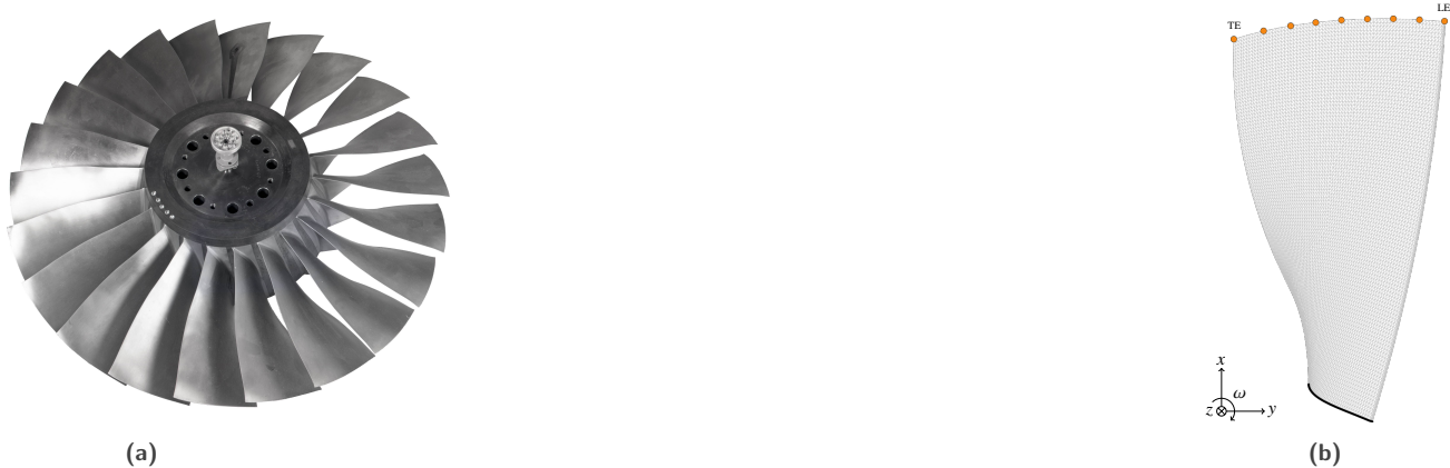
Figure 1. NASA rotor 67: (a) full blade disk [33], (b) finite element mesh with boundary nodes (●) [34]
