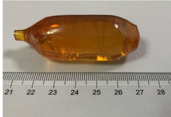
Figure. 1. Photograph of the as-grown 0.5 at.% Ho:CaY 0.9 Gd 0.1 AlO 4 crystal.
