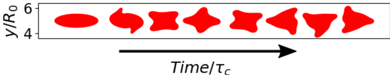
FIG. 3. Snapshots show the evolution of the vesicle shape from the initial configuration to the steady state. Here we set the confinement C_n = 0.2 , the capillary number C_a = 60.0 and the viscosity contrast \lambda = 7.0 (see movie 2 [64]). The steady state dynamic is shown in movie 1 [64].
