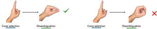
Figure 5: Depending on how participants perform thumb to finger tap to navigate the list during the disambiguation phase, the system would recognize the index as A) open or B) closed.
