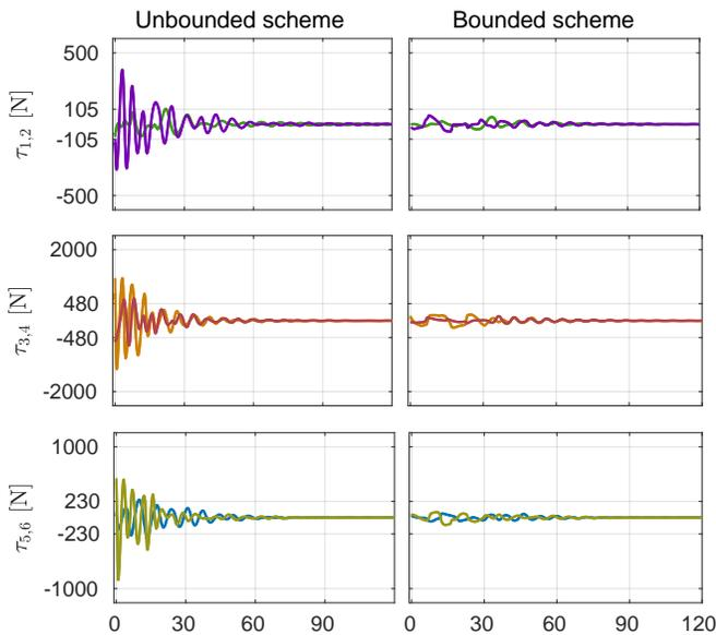
Fig. 6: Torque results for the unbounded scheme.
