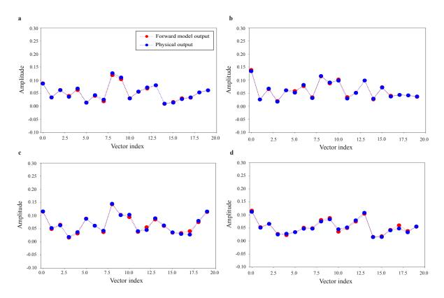
Figure S6 – Comparison of the forward model and physical microwave-PNN for four randomly selected inputs from the test dataset.
