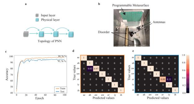
Figure 3 – Microwave-PNN. **a**, The topology of microwave-PNN consists of a three-layer PNN with skip connections. Each layer comprises a microwave-PNN augmented by trainable matrix multiplication. **b**, Photograph of the experimental setup. **c**, The train and test classification accuracy versus training epoch for the vowel recognition task. **d** and **e**, The confusion matrix for the PNN on the train and test set, respectively.
