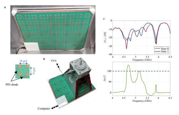
Figure S4 – **Details about the programmable metasurface. a**, Close-up view. **b**, Setup to characterize normal-incidence scattering properties of the metasurface. **c**, Normal-incidence characterization of the scattering response of the two different meta-atom configurations.
