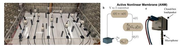
Figure S2 – Active control scheme and set-up photography a, Photography of the experimental set-up with the localization of the active nonlinear resonators. b, nonlinear active control scheme. c, Closed-up photography on the active nonlinear membrane (ANM).
