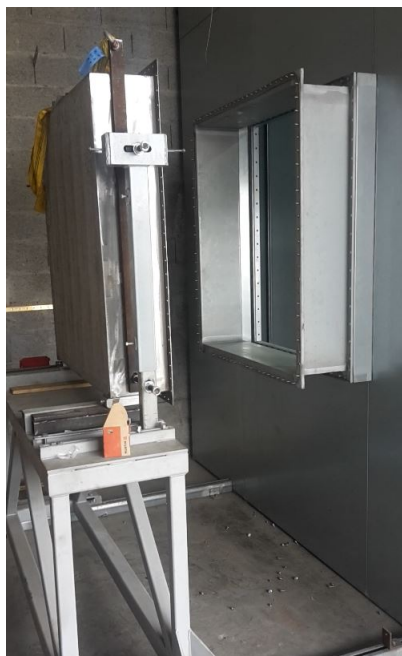
Figure 2: A fiber-reinforced concrete sample on its rolling cart, ready to be bolted on the square opening of the Faraday cage.
