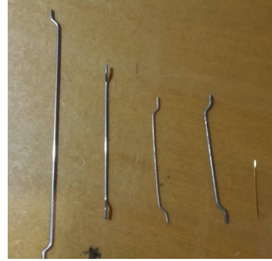
Figure 7: From left to right: fibers of type 80/60, 65/35, 80/30, 45/30 and 62/13.
