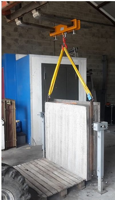
Figure 1: A fiber-reinforced concrete sample and its metallic frame.
