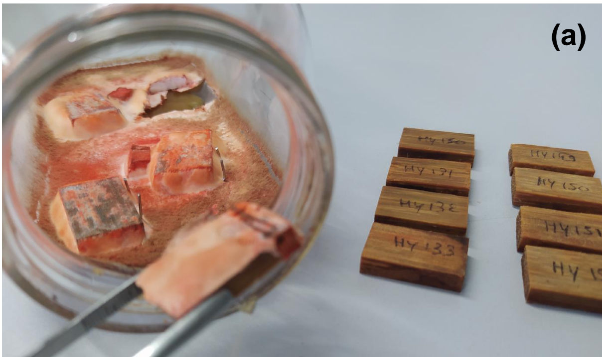
Cover picture. (a) Fungal and (b) termites laboratory screening tests carried out on 8 Guianese wood species. © Kévin Candelier
