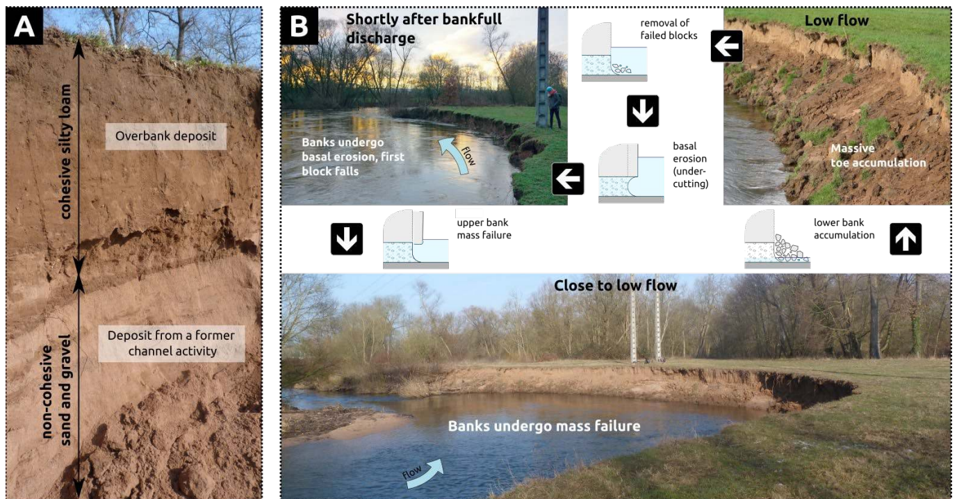
Fig. 14 – The cyclical process of bank retreat (Brierley and Fryirs, 2013) involved in the studied reach of the Lower Bruche.
