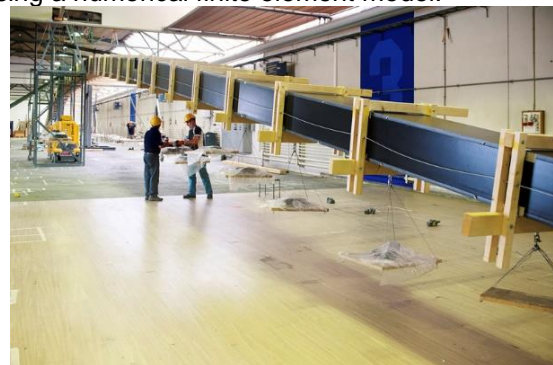
Figure 2: Wing load test of Solar Impulse 2 [3]
