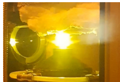
Fig. 9. Optical breakdown of droplets in an acetone spray/methane gas flame, \phi = 1.0 , v_{ex} = 1.73 m/s ( K \approx 347 s ^{-1} ).
