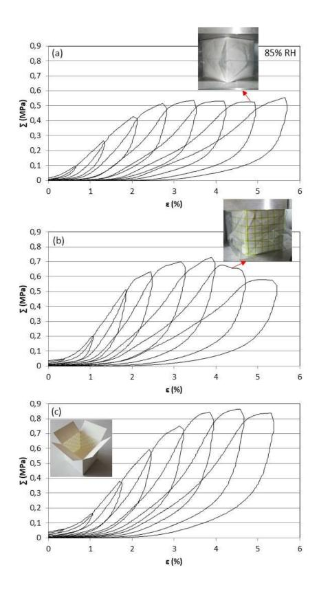
Figure 4. Loading and unloading evolution curves of (a) the reference (unprinted) box and of the boxes printed (b) on the outer side of the panels with the orthogonal grid and (c) on the inner side of the panels with the orthogonal grid orientated at 45°, with pictures of the boxes at different stages of compression.
