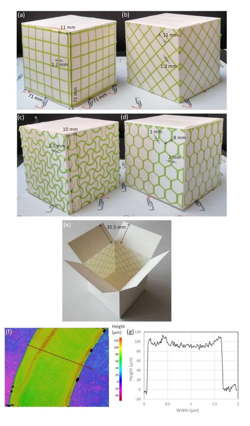
Figure 1. Pictures of boxes with panels printed on the outer surface with PLA-grid by FDM with the different patterns and their dimensions: (a) orthogonal, (b) orthogonal orientated at 45°, (c) sinusoidal and (d) honeycomb. (e) Picture of an opened box with panels printed on the inner surface. (f) Picture from the topographic measurement of the printed line of the sinusoidal pattern. (g) Evolution of the height of the printed line along its width (line represented in f).
