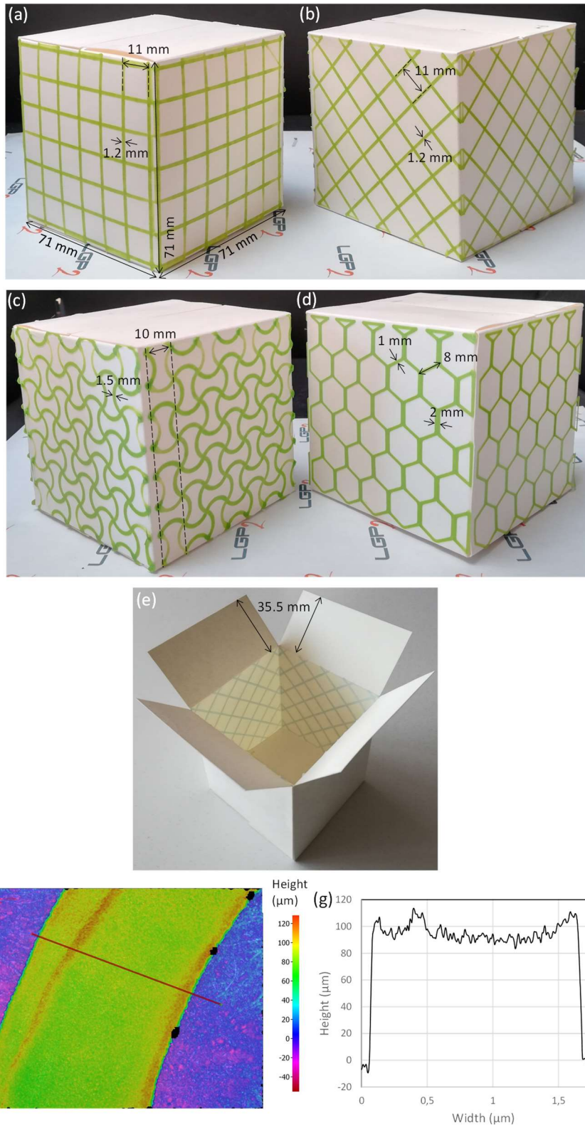
Figure 1. Pictures of boxes with panels printed on the outer surface with PLA-grid by FDM with the different patterns and their dimensions: (a) orthogonal, (b) orthogonal orientated at 45°, (c) sinusoidal and (d) honeycomb. (e) Picture of an opened box with panels printed on the inner surface. (f) Picture from the topographic measurement of the printed line of the sinusoidal pattern. (g) Evolution of the height of the printed line along its width (line represented in f).
