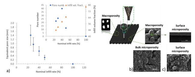
**Fig. 4.** a) Effect of the nominal infill during 3D printing on the size of macropores. Inset shows the pore number and the theoretical electrode material volume fraction in the infill mesh plotted as a function of the infill rate. SEM pictures of a) section of a 3D electrode on the ZY plane and b) surface of a dried unit filament.
