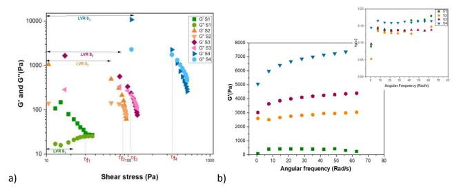
**Fig. 3.** a) Elastic and viscous modulus plotted as a function of the shear stress of the prepared samples  $(S_1, S_2, S_3, S_4)$  at a frequency of 1 Hz. b) Elastic modulus and loss angle's tangent (inset) plotted as a function of the angular frequency.
