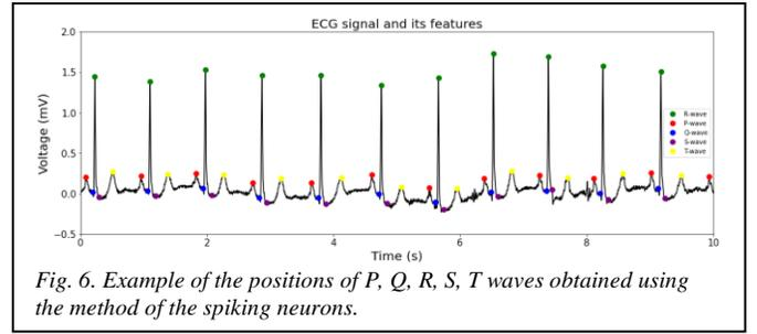
*Fig. 6. Example of the positions of P, Q, R, S, T waves obtained using the method of the spiking neurons.*
