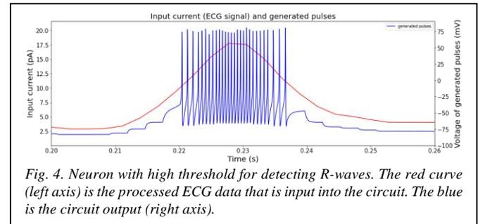
Fig. 4. Neuron with high threshold for detecting R-waves. The red curve (left axis) is the processed ECG data that is input into the circuit. The blue is the circuit output (right axis).
