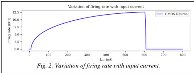
Fig. 2. Variation of firing rate with input current.
