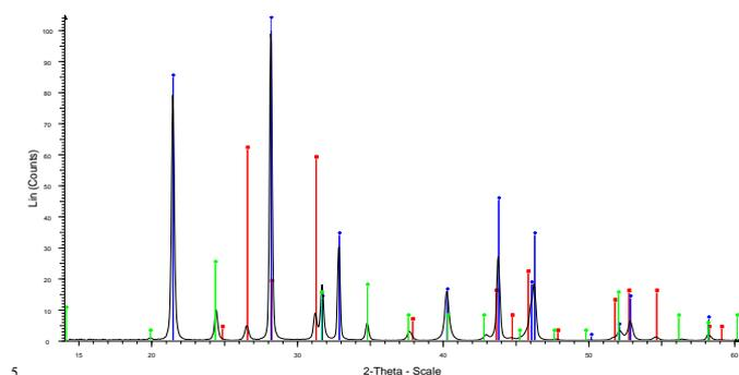
Fig 4: Diffractogram of a pellet after ageing 552 hours at room temperature in a tube containing 3mL of NaOCl (9.6%) and exposed to UV/Visible light. Red lines: cinnabar ( $\alpha$ -HgS), blue: calomel ( $\text{Hg}_2\text{Cl}_2$ ), green: corderoite ( $\alpha$ - $\text{Hg}_3\text{S}_2\text{Cl}_2$ ).
