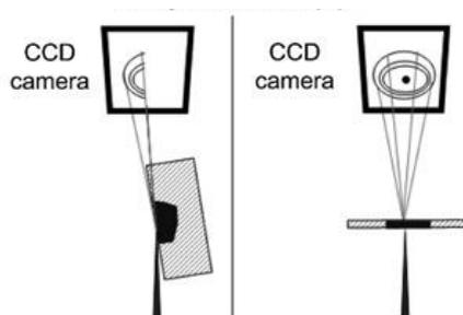
Fig 1: Reflection (left) and transmission (right) XRD geometry used resp. in the laboratory and SR-based  $\mu$ -XRD instruments.
