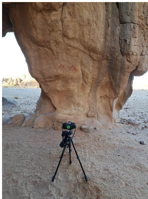
Fig. 4. The Specim IQ camera in the field measuring rock paintings.
