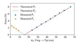
**Figure 3**. Theoretical – Eq. (1) – and measured right-hand finger forces against bow-string contact position, for a constant vertical string force  $F_S$  of about 1 N. Error bars are smaller than symbol size. Bow properties:  $x_{CM} = 29.6 \, \mathrm{cm}$ ,  $W_{bow} = 66 \, \mathrm{g}$ . Finger distances to pivot:  $x_I = 6.3 \, \mathrm{cm}$ ,  $x_L = 5.6 \, \mathrm{cm}$ .
