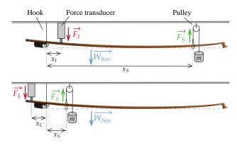
**Figure 4**. Setup for measuring static finger forces. Top: index finger (Fig. 3, squares). Bottom: little finger (id., circles).
