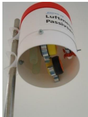
Figure 4.10 - LHS: Protective shelter for NH 3 Sampler; RHS: Mounting NH 3 Sampler with clips
