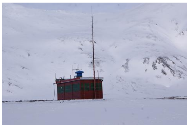
718 Figure 2: The environmental chamber facility of the PPSH, with various sampling heads exposed on 719 the roof in the spring 2019; a rainfall collector is located 100 m eastwards from there (Photo: K. Koziol)
