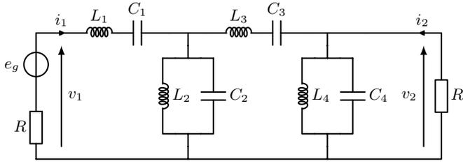
Fig. 2. A four-elements, LC-ladder bandpass filter
