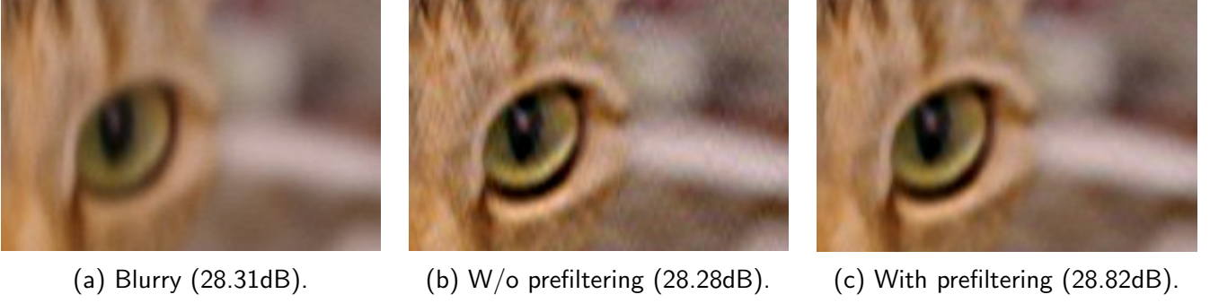
Figure 7: Qualitative comparison of the deblurred results after 3 iterations, but with and without the prefiltering technique based on [7]. The numbers in parenthesis are the PSNR scores computed with the original sharp image. The image is synthetically blurred, and further corrupted with Gaussian noise with \sigma_n = 0.01 and JPEG compression set to 85%. The variant of Polyblur without prefiltering magnifies the combination of noise and compression artifacts whereas with it, the image is deblurred and artifacts are kept with small magnitudes. The PSNR scores also indicate prefiltering helps to increase visual quality in presence of noise/compression artifacts.
