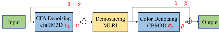
FIGURE 3. Generic raw image processing pipeline. This pipeline structure allows for an arbitrary order between DN and DM and sets free their parameters. We use the CMA-ES algorithm to optimize the parameter \alpha , \beta , \sigma_1 , \sigma_2 in the pipeline.
