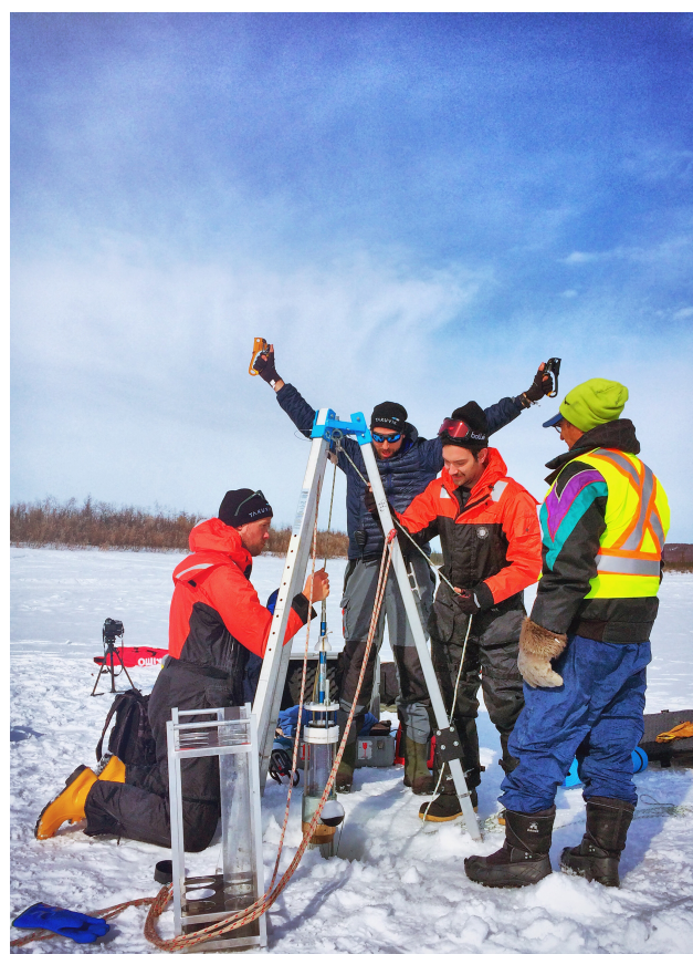
Figure E1. Picture taken during Leg 1 of the Nunataryuk expeditions showing the setup of the tripod and corer (picture credit: Martine Lizotte).
