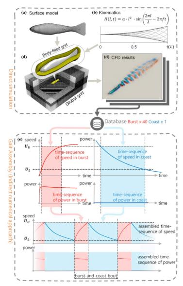
**FIG. 2.** Numerical methods. (Upper) Direct numerical approach: (a) Fish surface model; (b) Kinematic model; (c) Computational mesh; (d) An example of CFD flow field; (e) Indirect numerical approach: Burst-and-coast *gait assembly*.
