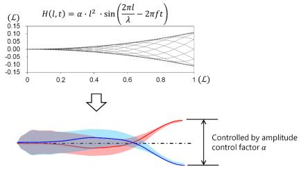
Deformation in a reference frame attached to fish head
