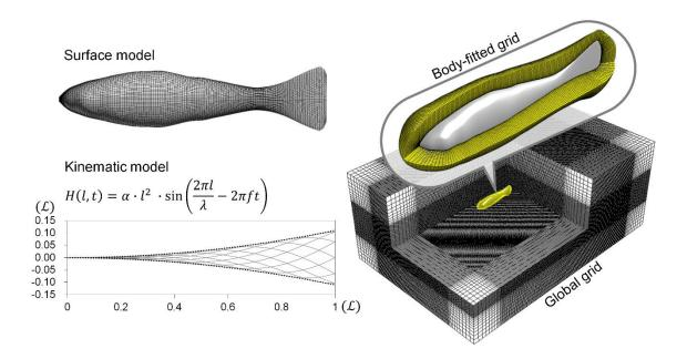
**Figure S2**. Computational fluid dynamics model. (a) Surface model of Red nose tetra fish (dimension: 97×121); (b) A function drives the instantaneous body shape. Variation of body length caused by this driving function was corrected to keep lateral excursion and body length constant at 1*L*. (d) Multi-blocked computational grid system consists of local fine-scale body-fitted grid (dimension: 97×121×20 at Re<1000, 97×121×60 at Re>1000) plus a large stationary global grid (dimension: variant).
