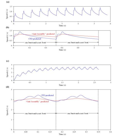
**Table S8.** Comparison between CFD and "gait assembly" speed results. (A) Speed curve of CFD Case 1; (B) Comparison of speed curves between CFD and "gait assembly" at 1L/s; (C) Speed curve of CFD Case 2; (D) Comparison of speed curves between CFD and "gait assembly" at 3L/s.
