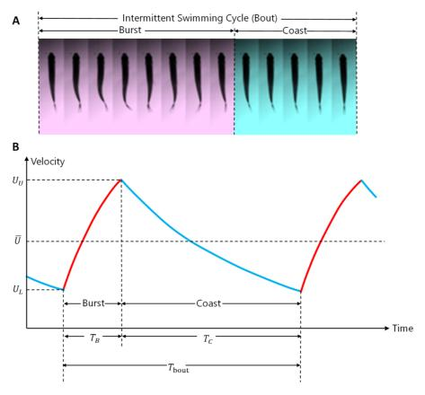
**FIG. 1.** Features of burst-and-coast swimming. (a) Example observation on burst-and-coast swimming; (b) Schematic description of burst-and-coast swimming with regards to time and velocity, redrawn from Videler and Weihs [10].
