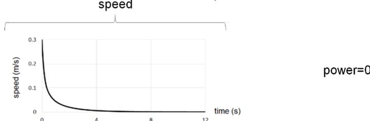
**Fig. S7** Simulated time-sequences of speed and power, respectively in 40 full burst processes and one coast process.  $f$  is tail beat frequency and  $\alpha$  is the tail beat amplitude control factor, the non-linear relation between amplitude  $A$  and  $\alpha$  is shown in Table S3
