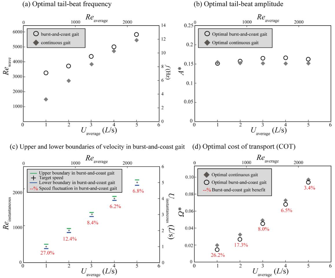
**FIG. 6.** Comparison between optimal burst-and-coast and continuous gaits at various speed levels. (a) optimal tail-beat frequency; (b) Optimal tail-beat amplitude; (c) Upper and lower speed boundaries of optimal burst-and-coast swimming, and the fluctuation range around the average speed. Note that upper and lower velocity boundaries are not applicable for the continuous gait; (d) Cost of transport of optimal burst-and-coast gait and continuous gait.  $1L/s = 0.02m/s$ .
