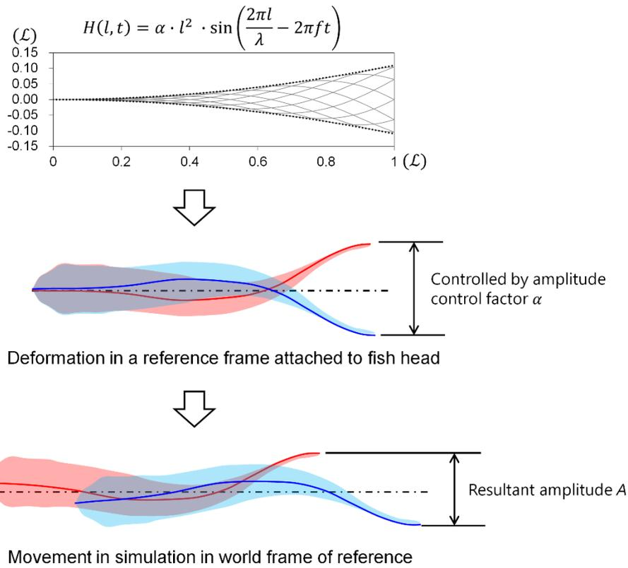
**Figure S5.** We defined the model fish tail motion in a reference frame attached to the fish, while the resultant fish tail motion ('emerging' from the simulation) in a world reference frame is influenced by recoil (i.e., overall body rotation) and becomes narrower.
