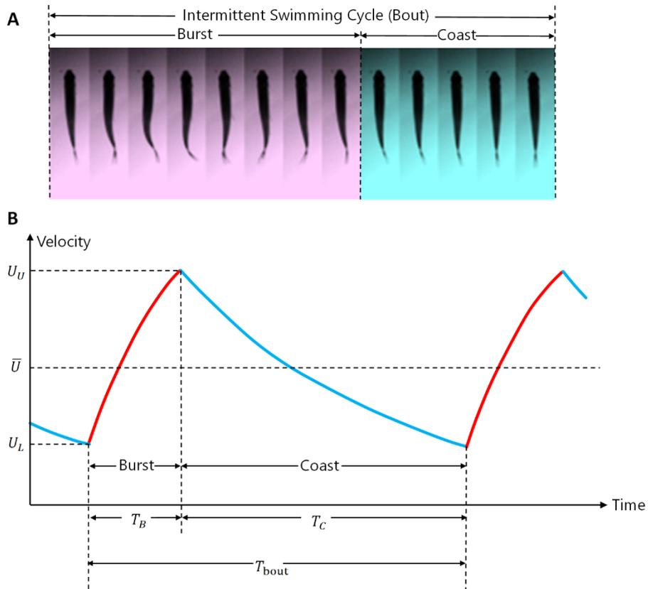
**FIG. 1.** Features of burst-and-coast swimming. (a) Example observation on burst-and-coast swimming; (b) Schematic description of burst-and-coast swimming with regards to time and velocity, redrawn from Videler and Weihs [10].
