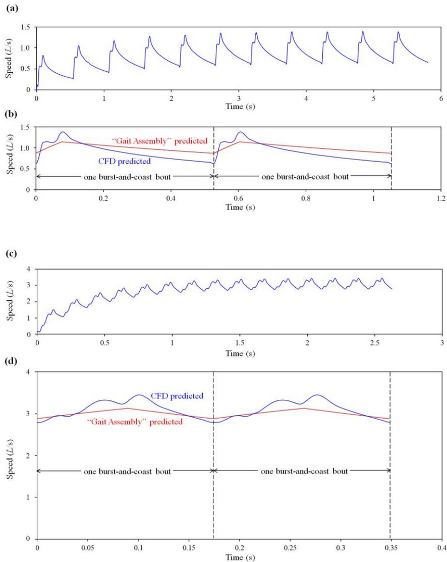
**Table S8.** Comparison between CFD and "gait assembly" speed results. (A) Speed curve of CFD Case 1; (B) Comparison of speed curves between CFD and "gait assembly" at 1L/s; (C) Speed curve of CFD Case 2; (D) Comparison of speed curves between CFD and "gait assembly" at 3L/s.
