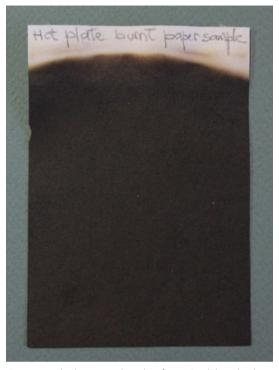
Fig. 3. Paper samples burnt on a hot plate for testing (Photo by the author)
