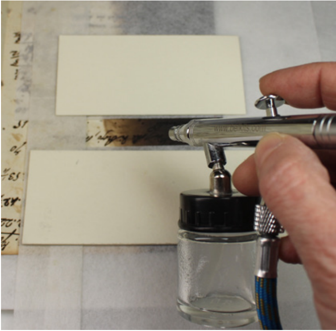
Fig. 7. Distribution of the nanocomposite formulation by airbrush on the charred area of a manuscript (Photo by the author)
