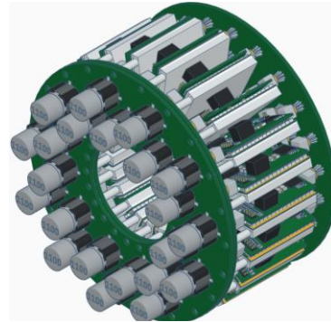
Fig. 15 3D CAD of the designed IMMD for the OW-PMSM.
