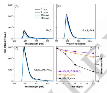
Figure 3. Evolution of the PL spectra with time after synthesis (after 0, 7, 15, and 30 days) of (a)  $Ga_2S_3$  core, (b)  $Ga_2S_3/ZnS$  core/shell, and (c)  $Ga_2S_3/ZnS/Al_2O_3$  core/shell/shell QDs. (d) Temporal evolution of PLQY relative to the starting value just after synthesis.
