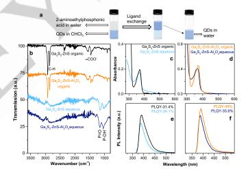
Figure 6. Schematic representation of the aqueous phase transfer of the core/shell and core/shell/shell QDs. (b) FTIR, (c) Absorption, (c) PL spectra of Ga<sub>2</sub>S<sub>3</sub>/ZnS and Ga<sub>2</sub>S<sub>3</sub>/ZnS/Al<sub>2</sub>O<sub>3</sub> QDs before and after phase transfer ligand exchange.
