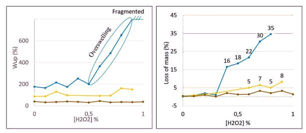
Figure 2: Evolution of water uptake (left) and loss of mass (right) of sPEEK\_NS membrane (blue), HTU 6.5%SG (yellow) and 28.6%SG (brown) depending on the degrees of exposition to H<sub>2</sub>O<sub>2</sub>
