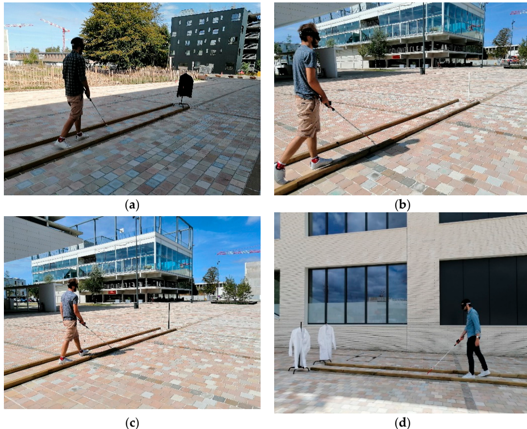
Figure 3. A sighted blindfolded participant sweeping the cane between the two bars at a given cadence to detect (a) a large dark obstacle under intermediate luminosity conditions; (b) a white thin post in full sunlight; (c) a dark thin post in full sunlight and (d) an aperture.
