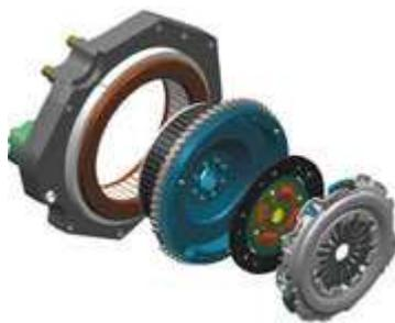
**Fig. 7** Exploded view of the IPMSM (stator and rotor on the left) and the clutch system
