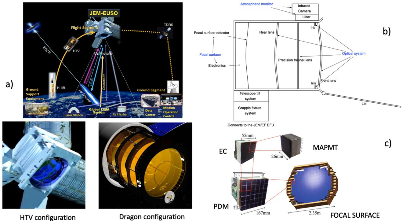
**Fig. 1** Panel a: Conceptual view of the whole JEM-EUSO system. Panel b: Conceptual design of the JEM-EUSO system: three Fresnel lenses focus the light on the focal surface. Panel c: Conceptual design of the JEM-EUSO Focal Surface with its elements and sub-elements parts. The focal surface of the detector is formed by 137 Photo Detector
