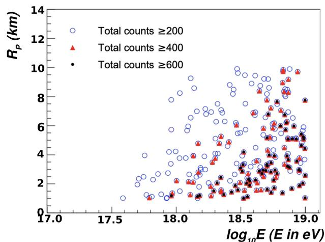
**Fig. 37** Relation between the EAS energy and the impact parameter  $R_p$ . 1000 proton events were simulated, and among them 229, 118, and 67 events generated more than 200, 400, and 600 counts over 3 consecutive GTUs in the EUSO-TA detector, respectively. In this plot a cosmic ray power spectrum  $E^{-1}$  has been considered: more events at high energies are present in the plot than expected in reality, for which the average spectrum scales by about  $E^{-3}$ . Image taken from [98]
