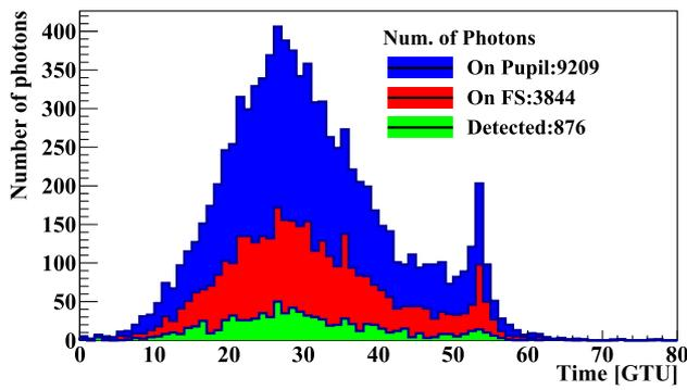
**Fig. 12** Photons coming to the detector, photons intersecting the focal surface (FS) and photons detected as a function of time (in GTU). Due to the covering factor and quantum efficiency taken into account, the fraction of photons creating a signal (‘Detected’) is about 0.3. In this example:  $10^{20}$  eV proton event with  $60^\circ$  zenith angle
