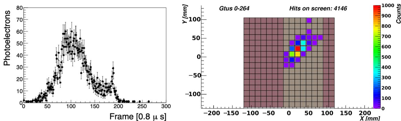
**Fig. 21** A simulated  $10^{21}$  eV,  $60^\circ$  zenith angle proton event. Left panel: The photoelectron profile for the TUS detector. Right panel: The photoelectron image for TUS. Image taken from [80]
