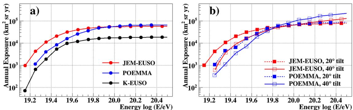
**Fig. 13** JEM-EUSO, K-EUSO and POEMMA exposures as a function of energy for nadir (left) and different tilting angles (right). In case of K-EUSO only the nadir configuration has been simulated as the tilt option is not considered in the present mission design
