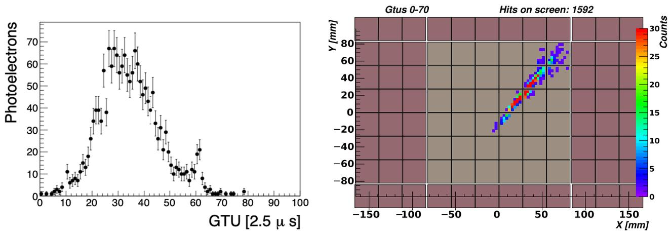
**Fig. 20** A  $10^{20}$  eV,  $60^\circ$  zenith angle proton EAS. On the left: The photoelectron profile for the POEMMA detector. On the right: The image on the POEMMA’s focal surface. Image taken from [80]
