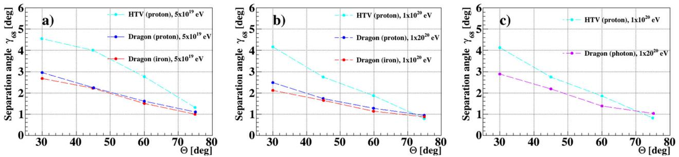
**Fig. 15** The angular resolution as a function of the zenith angle for the Dragon-configuration of the JEM-EUSO mission pointing to nadir for proton (dark blue) and iron (red) primaries with an energy of  $5 \times 10^{19}$  eV
