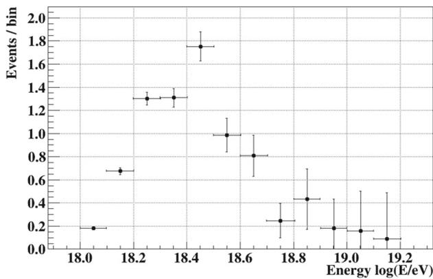
**Fig. 31** The expected number of triggered EAS for EUSO-SPB1 floating at an altitude of 30 km assuming clear sky condition and a flight duration corresponding to 118 h of dark time. Image adapted from [92]
