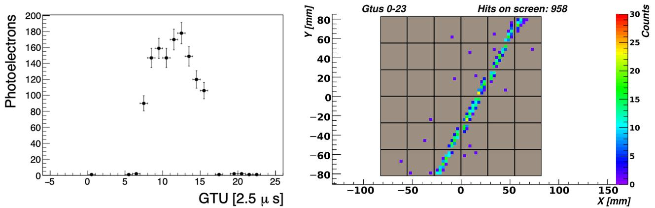
**Fig. 35** A  $10^{19}$  eV,  $45^\circ$  zenith angle simulated proton event impacting at 25 km distance from the detector. Panel a: The photoelectron profile for the EUSO-TA detector. Panel b: The photoelectron image for EUSO-TA. Image taken from [80]
