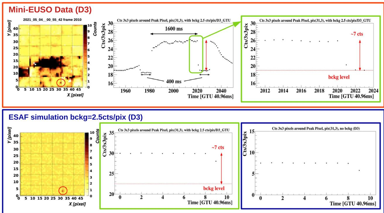
**Fig. 28** Top: Mini-EUSO flasher campaign event. The central panel shows the light evolution of summed counts of  $3 \times 3$  pixels around the peak count pixel, indicated by the red-circle on the left plot, for a cycle of 1600 ms pulse (GTU = 40.96 ms). The transit of the 1600 ms pulse preceded and followed by 400 ms off is clearly seen. Right panel: The zoomed in plot to the duration and timing where ESAF simulated the same event, as shown in the bottom plots. Bottom: Simulated flasher
