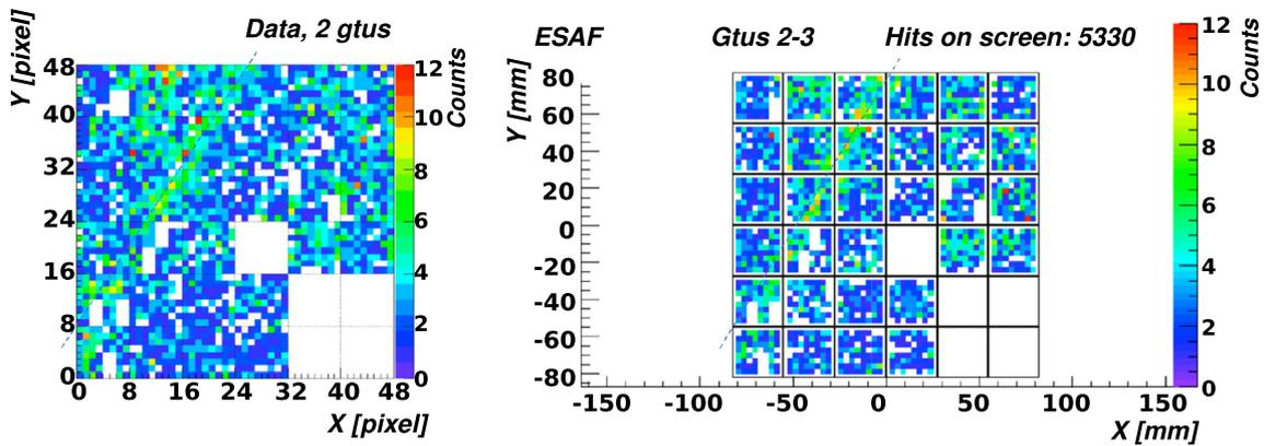
**Fig. 36** Comparison between an UHECR event observed by EUSO-TA (left) and a proton shower simulated with ESAF (right) assuming the EAS parameters provided by the TA reconstruction of the event ( $E = 2.4 \times 10^{18}$  eV, zenith  $\theta = 41^\circ$ ). No longitudinal distribution is provided for this event as its duration is confined in 2 GTUs. The back-
