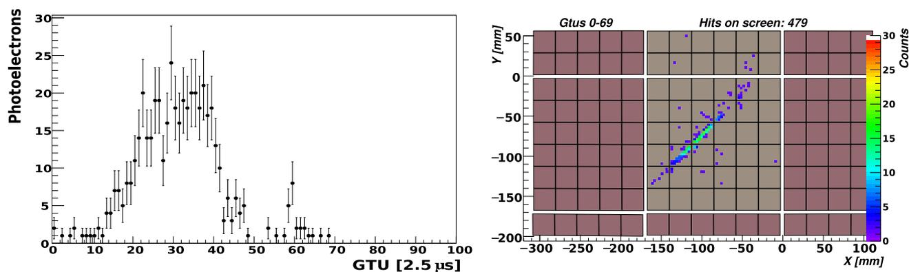
**Fig. 8** Simulation of a  $10^{20}$  eV,  $60^\circ$  zenith angle proton event performed for one of the proposed and studied configurations of the K-EUSO detector. On the left, a photoelectron profile at the focal surface is shown. The photoelectron image of the same event on the FS is shown in the right panel
