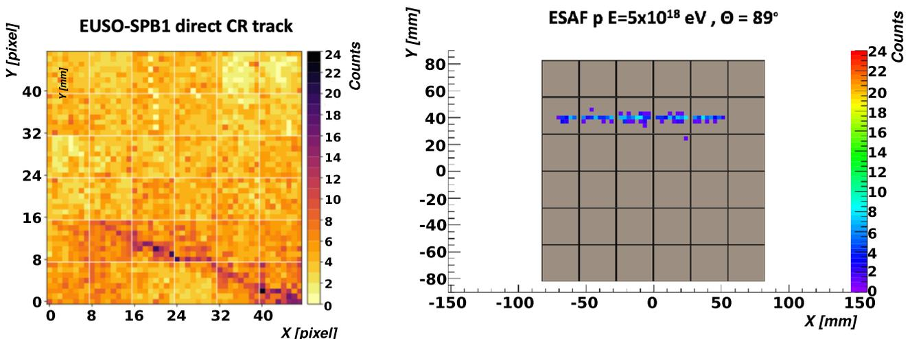
**Fig. 32** Left side: Direct cosmic ray triggering the EUSO-SPB1 detector. Right side: Simulated proton EAS of energy  $E = 5 \times 10^{18}$  eV crossing the balloon FoV at  $\sim 25$  km altitude with a zenith angle of  $\theta = 89^\circ$ . They both correspond to 1 GTU data
