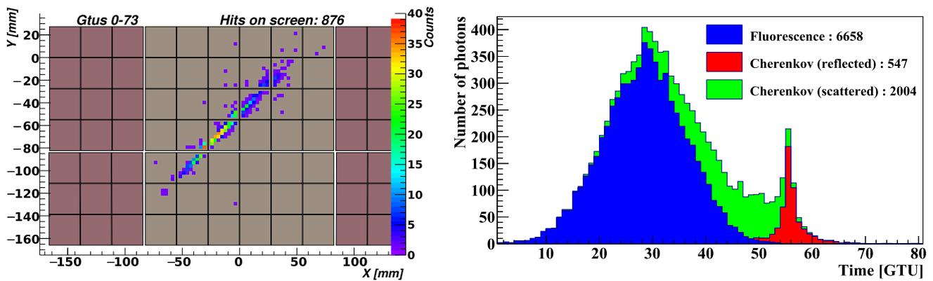
**Fig. 11** Left: Spatial profile of photon counts from an EAS caused by a  $10^{20}$  eV proton with zenith angle  $60^\circ$ . Each square (dark and light brown) represents a MAPMT. Parts of 6 PDMs are shown. The small coloured squares show the number of photon counts detected by each channel of the MAPMT. This event is crossing two PDMs, with the shower starting to develop in the bottom central PDM and continuing in
