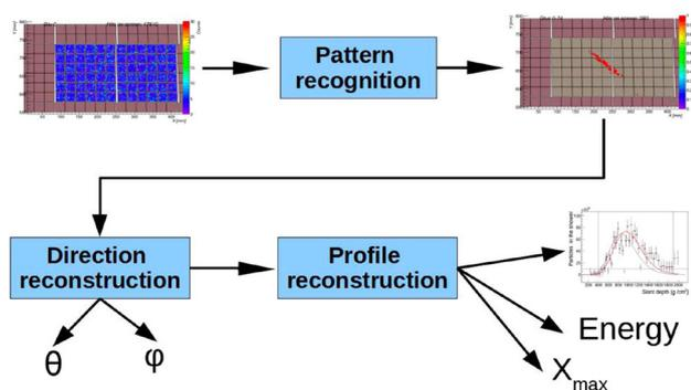
**Fig. 9** The general scheme of the reconstruction framework
