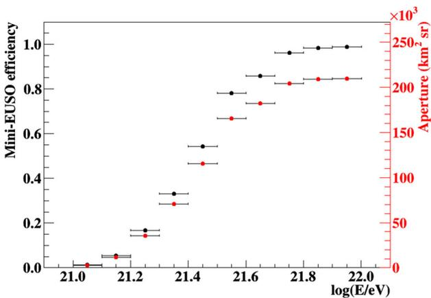
**Fig. 24** The trigger efficiency (on the left axis, in black) and geometrical aperture (on the right axis, in red) are shown as a function of the EAS energy,  $E$ , in eV. A UV background level of 1 count/pixel/GTU( $2.5 \mu\text{s}$ ) was considered in both cases
