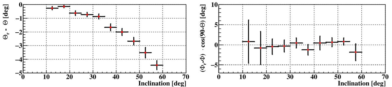
**Fig. 34** Mean value and standard deviation of  $\Delta\Theta = \Theta_{rec} - \Theta_{sim}$  (left) and  $\Delta\Phi = (\Phi_{rec} - \Phi_{sim}) \cos(90 - \Theta)$  (right) plotted against the true zenith angle (inclination) for EUSO-Balloon. Image adapted from [97]
