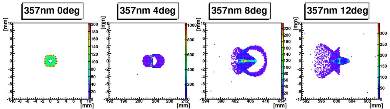
**Fig. 7** PSF diagrams of one version of the K-EUSO optics. Panels correspond to light at 357 nm with incident angles from the optical axis  $0^\circ$ ,  $4^\circ$ ,  $8^\circ$  and  $12^\circ$  respectively. The size of each frame is  $20 \text{ mm} \times 20 \text{ mm}$ .
