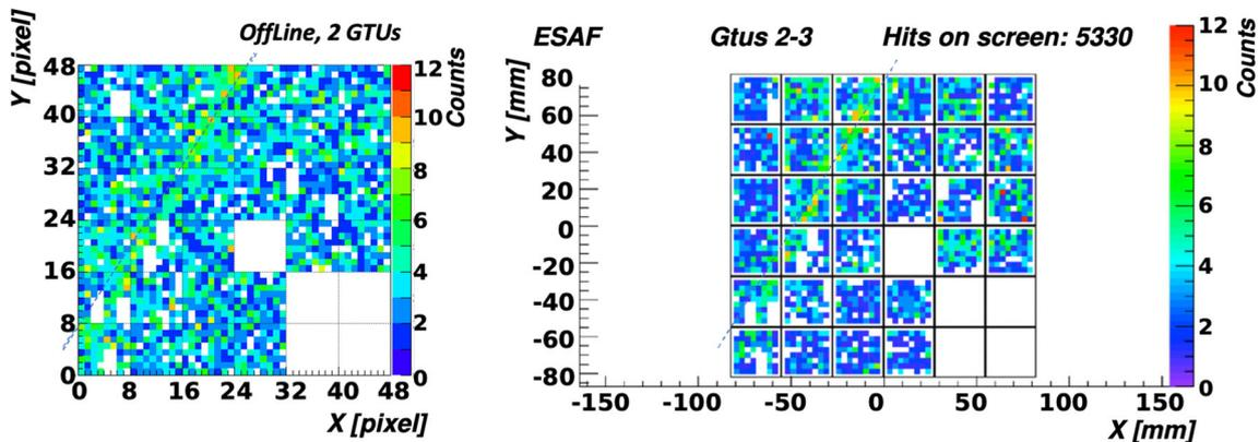
**Fig. 40** Comparison between a proton shower simulated with OffLine (left) and ESAF (right) assuming the EAS parameters provided by the TA reconstruction of the event ( $E = 2.4 \times 10^{18}$  eV, zenith  $\theta = 41^\circ$ ) shown on the left side of Fig. 36
