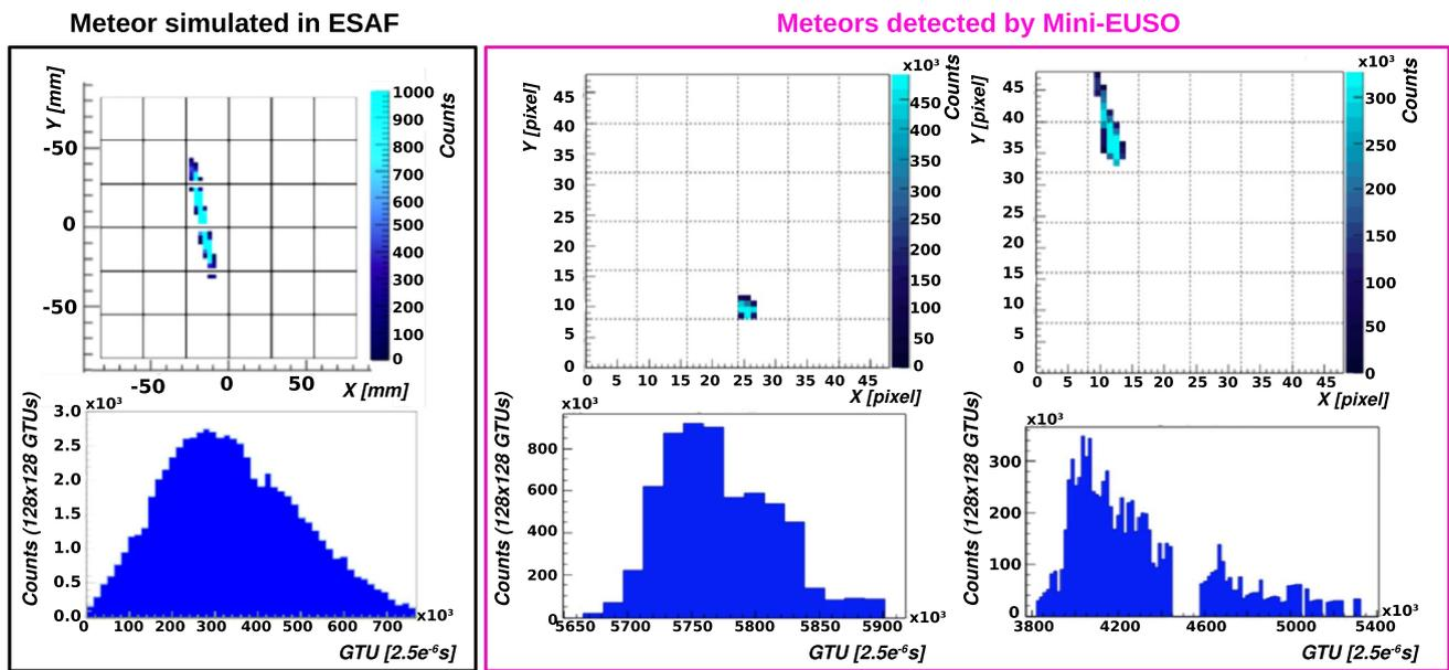
Fig. 26 Left panel: ESAF simulated light track of a meteor of absolute magnitude  $M = +5$  and  $45^\circ$  inclination in Mini-EUSO (the effects of UV-nightglow are not included and the threshold is 30 counts). Bottom: Expected light profile. Each time bin on the x-axis corresponds
