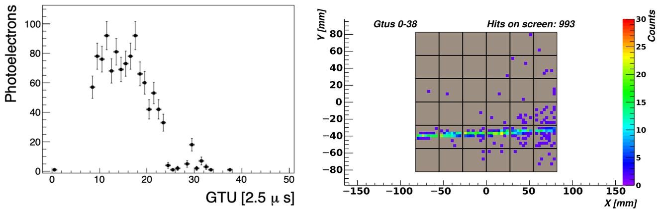
**Fig. 29** A  $10^{19}$  eV,  $45^\circ$  zenith angle simulated proton event. Left: The photoelectron profile for the EUSO-SPB1 detector. Right: The photoelectron image for EUSO-SPB1. Image adapted from [80]
