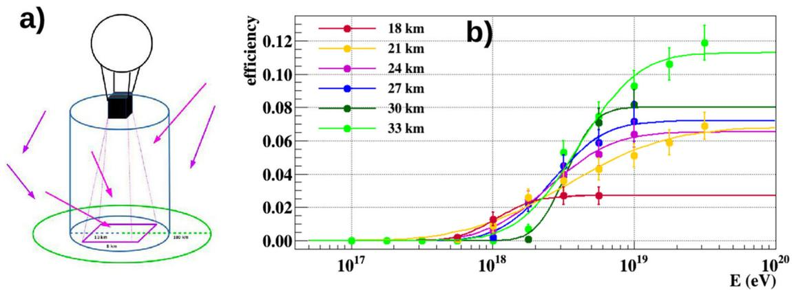
**Fig. 30** Panel **a**): To speed up the simulation process in balloon configurations, EASs are fully simulated if crossing a cylindrical volume  $\mathcal{V}$  which includes the balloon FoV. EAS not crossing this volume are
