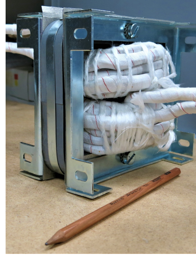
Figure 2: MFT prototype made with two high temperature 10 turns coils.
