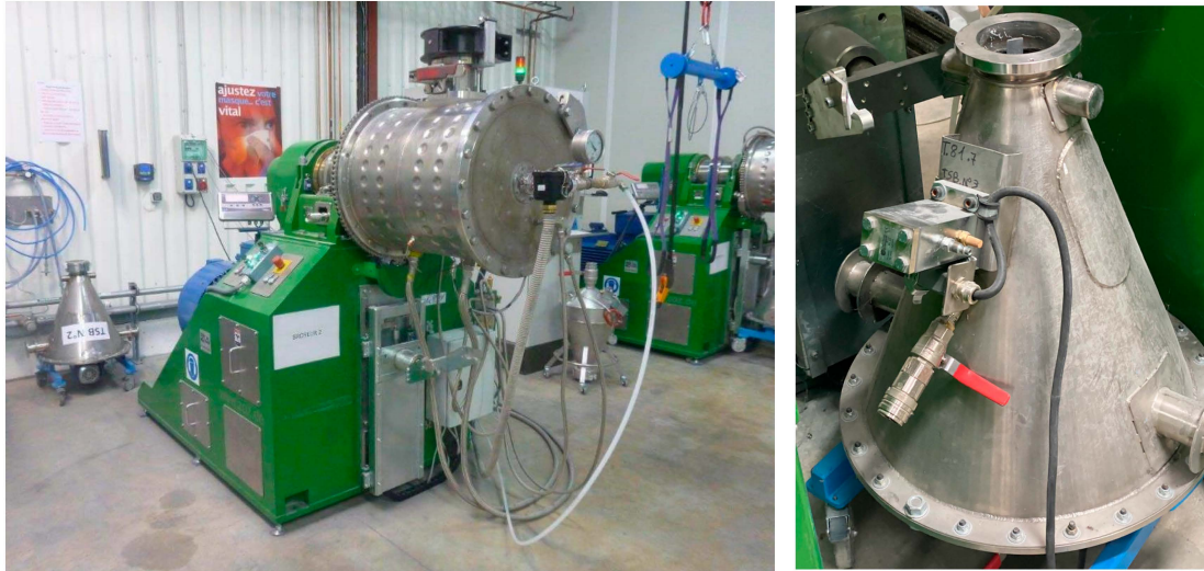
Figure 2. Left: Ball-millers, with aside a transfer container; Right: Details of a transfer container.
