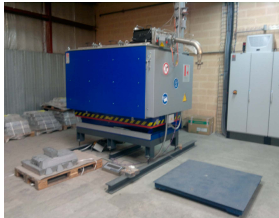
Figure 8. The CPM smelter (Rauch GmbH, Gmunden, Austria) equipped with a proboscis to pump and flow the melt in the specific volume of the dual tank to be installed on the torque in front of the smelter. This enables distribute the exact amount of CPM necessary to store heat involved at the exo-(endo-) thermal \text{Mg} \leftrightarrow \text{H}_2 reactions.
