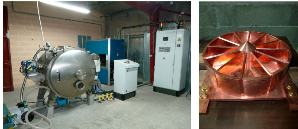
Figure 4. Left—HF induction equipment to prepare metal-type additives, Right—the casting mold.
