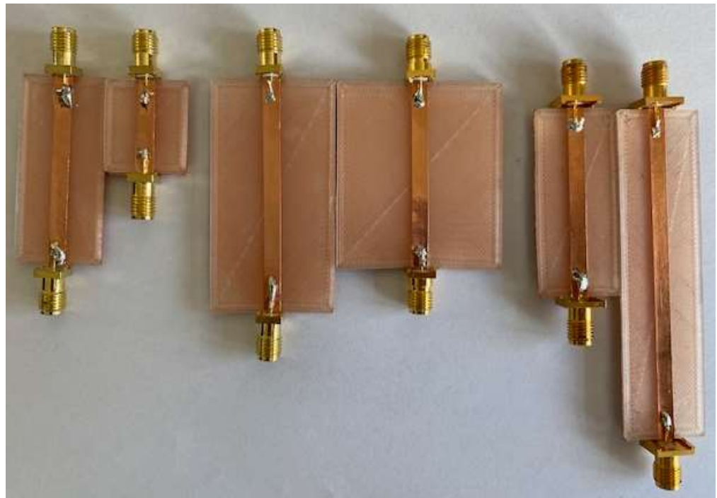
Figure 2. Three-dimensional FDM-printed substrate transmission lines with copper tape.
